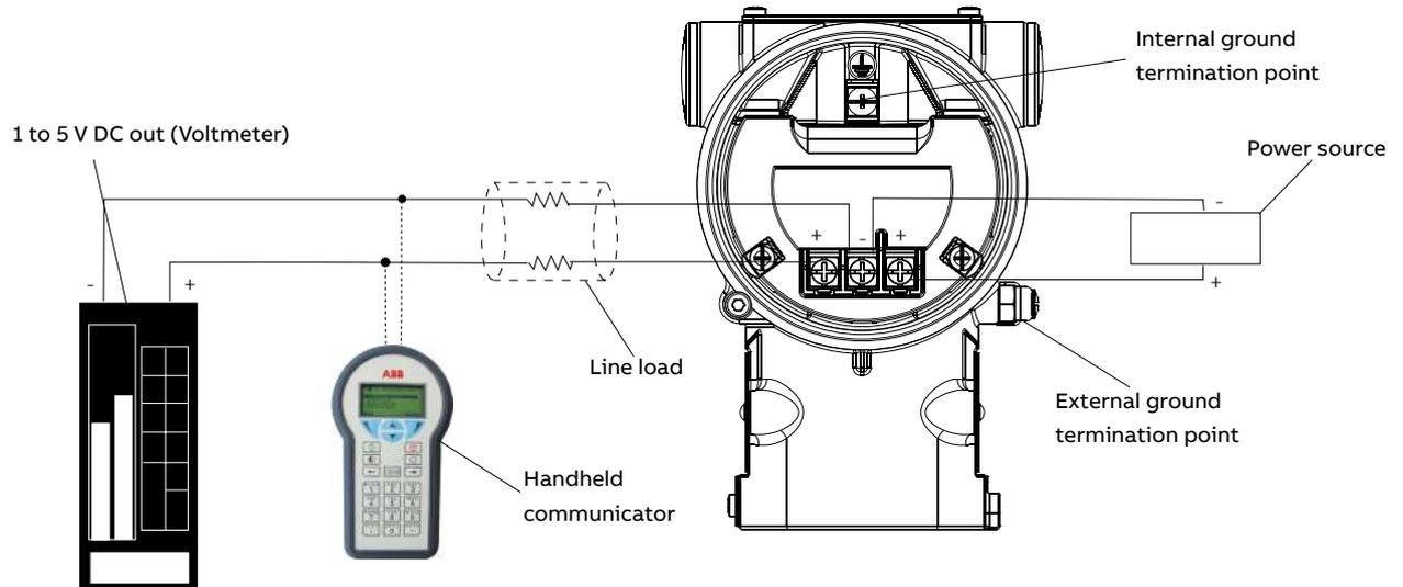
HART handheld communicator may be connected at any wiring termination point in the loop, providing the minimum resistance is 250 ohm. If this is less than 250 ohm, additional resistance should be added to allow communications.
