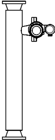
STYLE 1 TOP AND BOTTOM CONNECTIONS, SCREWED (S-1) OR FLANGED (F-1)
