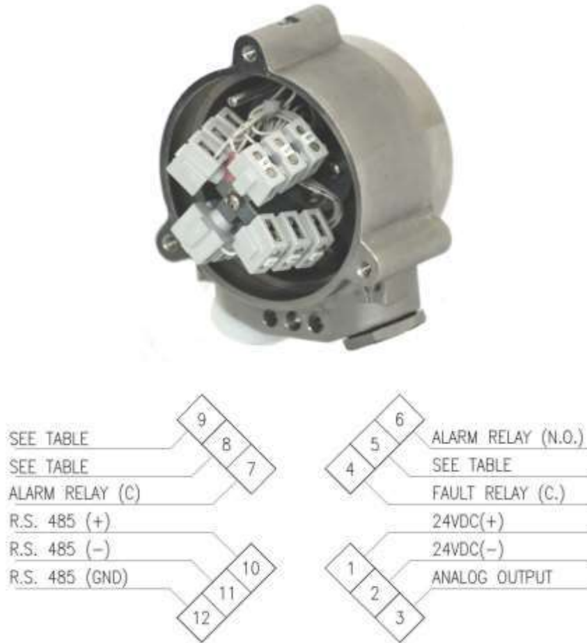
Figure 8: Wiring Terminals
